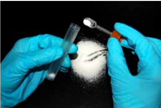
Sterile scoop with inner tube, sample over-packed in a 50 ml centrifuge.
